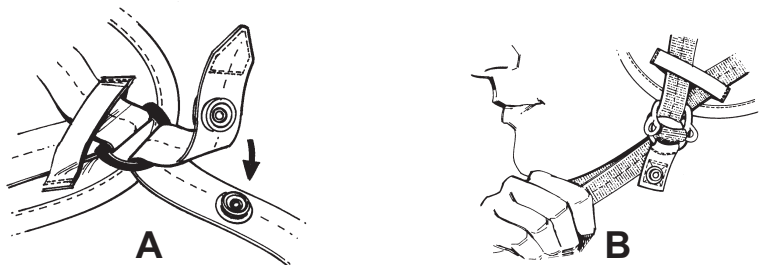
Figure 5. Fastening and Adjusting Chinstrap
