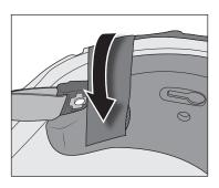
Re-attach the Fitband to the Front EPP Pad.
