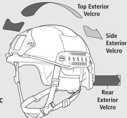
**\*ALL DIAGRAMS ARE SHOWING THE FAST BALLISTIC HIGH CUT HELMET. YOUR HELMET SHELL AND VELCRO PATTERN MAY VARY.**
