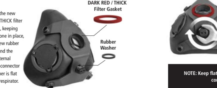
**NOTE:** Keep flats on locknut and the two round electronic connectors horizontal as shown.
