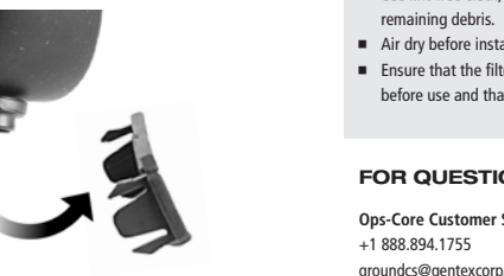
2 Replace with a CR123 battery as shown and reattach the battery cover.
