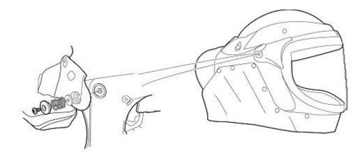
Replace an old or damaged visor on Pureflo 50ESM+ (P-Series) Pharmaceutical bump cap variant as per instructions below:
